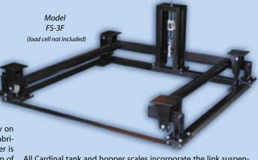
All Cardinal tank and hopper scales incorporate the link suspension bearing system. Link suspension bearings absorb impacts and provide a free-floating platform. The levers are constructed of structural steel shapes and extra heavy seamless steel tubing to give greater strength than much heavier materials of comparative low tensile strength.
