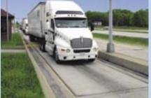
Modules may be marked with a painted edge stripe to assist the driver in properly positioning the truck. Each section functions as an independent scale.
