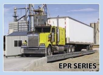
Cardinal's EPR Series truck scales utilize an interlocking yoke and pin, "No Bolt" assembly. Installation is simple - just assemble the modules in place, then install the load cells and suspension assemblies. The low-profile design allows easy access to the load cells and wiring, making installation and maintenance a snap.
