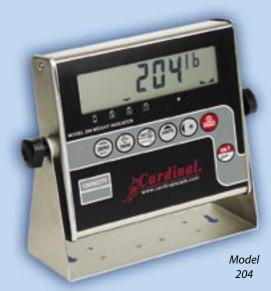
Dimensions: 8" W x 2.125" D x 6.625" H (20 cm W x 5 cm D x 17 cm H) Enclosure: NEMA 12/IP55 stainless steel Resolution: 5,000 divisions Power: 115 VAC 60 Hz adapter or, 230 VAC 50/60 Hz, or 6 "C" cell alkaline or rechargeable Ni-Cad batteries Load Cells: Up to 4, 350 ohm Keyboard: 7 keys Units Conversion: Pounds, kilograms, grams,
